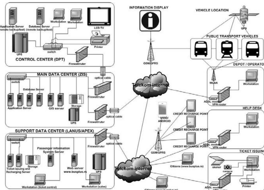
Fig. 1. The system's architecture in Belgrade
