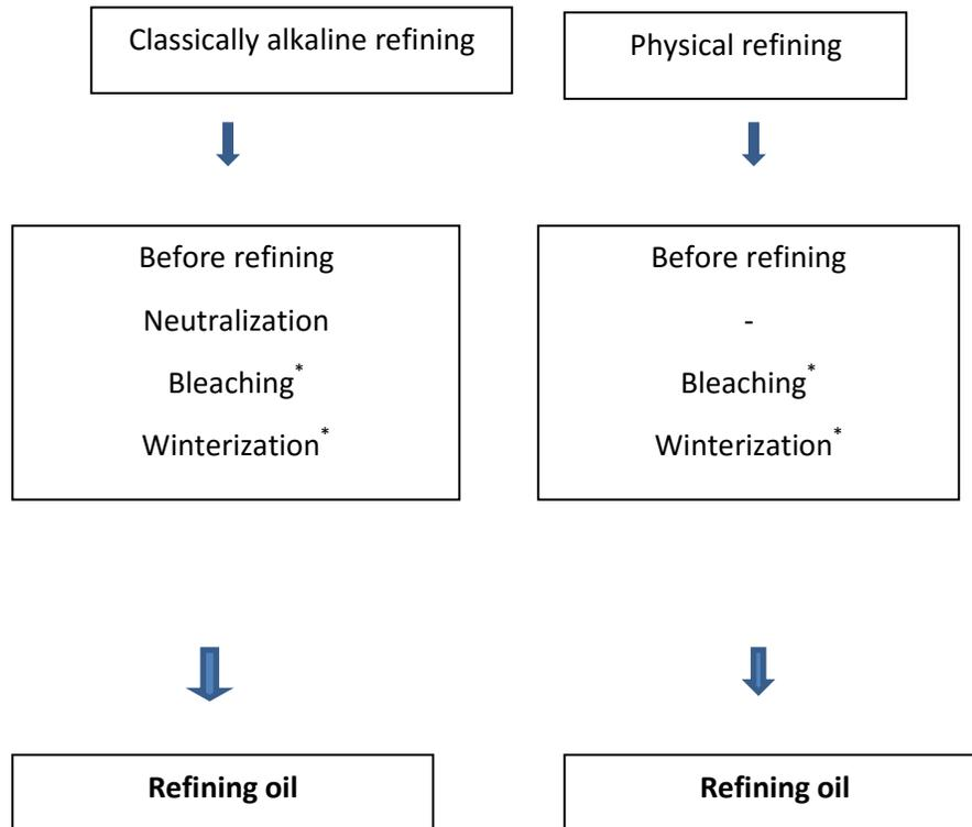
Scheme 1. Technological scheme of obtaining raw and refined oil [3]
